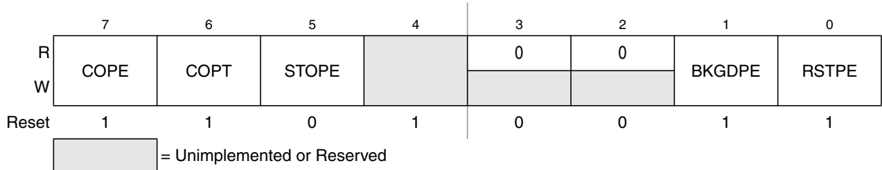
Figure 5-5. System Options Register (SOPT)
